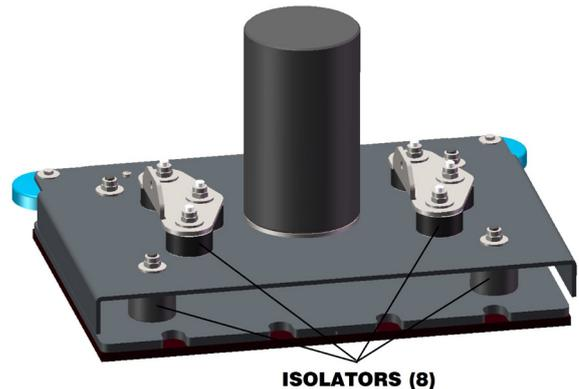
2. If any of the eight isolators show signs of wear, degradation or damage, contact your local distributor to replace all eight isolators.
